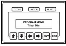
The minimum run timer defines the minimum amount of time a tool has to run during a fastening process in order to be considered a good fastening. If a fastening process is shorter than timer min, a Tmin reject will be issued.
