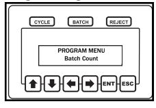
The Batch Count is typically programmed to be the number of fasteners in a given assembly. A Cycle Accept signal will be generated each time a proper fastening occurs. A Batch Accept however, will occur when the count reaches the
