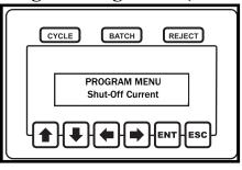
The shut-off current defines the minimum amount of current that needs to be drawn by a brushless tool when the tool clutches out. This threshold can be used as a secondary check for the tool's clutch setting. The shut-off current value is only used with brushless tools.
