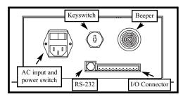
The rear panel on the unit contains several items. The main power switch for the unit and the power entry module are found on the back panel. This unit is capable of running on an
