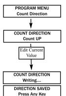
display reads PROGRAM MENU, Count Direction. Press the enter button in order to edit the Count Direction.
