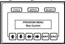
The maximum current defines the maximum amount of current that can be drawn by a brushless tool when the tool clutches out. This threshold can be used as a secondary check for the tool's clutch setting. **The max current value**
