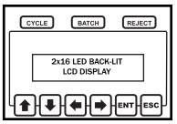
A two line by sixteen character back-lit LCD display is part of the user interface. This display will provide the user with feedback during the run mode and guide the user through programming functions.
