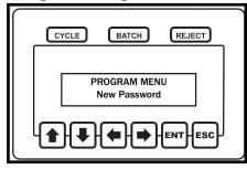
In order to enter the programming mode, either the keyswitch was used or a password was entered. The default password of 0104 can be overwritten and set to any four digit number.
