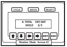
The second monitor screen shows current parameter, total batches completed, current count, and number of fasteners in a batch.
