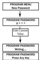
In order to change the password, enter the program mode and press an arrow key until the display reads PROGRAM MENU, New Password. Press the enter button in order to edit the password.
