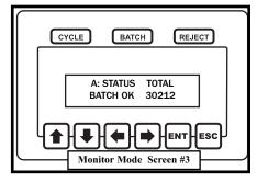
The third monitor screen shows current parameter, status of the last fastening, and total number of fasteners in the batch.
