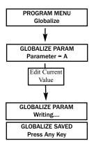
is the case, globalizing a parameter set may help to speed the programming process. When globilization is used one parameter set is copied to all of the other parameters.
