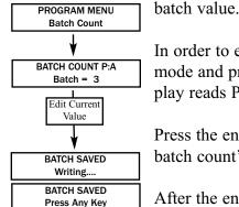
In order to edit this value enter the program mode and press an arrow key until the display reads PROGRAM MENU, Batch Count.
