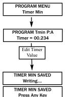
In order to edit this value enter the program mode and press an arrow key until the display reads PROGRAM MENU, Timer Min.
