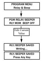
The beeper in this system can be programmed to double-beep when a batch accept occurs.
