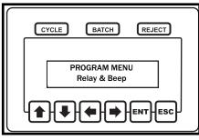
The output relays in this system can be programmed to be either momentary or latching. If the relays are momentary the will close briefly (200ms) when and event occurs. When set to latching, the relay closes and remains that way until the tool starts running again.
