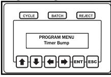
The bump timer defines an amount of time that a tool can run and that run will be ignored if the clutch does not fire (i.e. torque is not achieved). This timer may be used to eliminate nuisance rejects.
