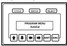
The first item on the program menu is AutoCal<sup>TM</sup>. AutoCal<sup>TM</sup> is a calibration routine that is meant to get the unit up and running very quickly. In order to use the AutoCal<sup>TM</sup> feature press the enter button.
