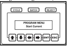
The start current defines the amount of current that needs to be drawn by a brushless tool before the unit is considered to be in cycle. Once the tool starts drawing this amount of current, the run-timers will start. The start current value
