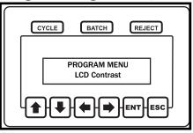
The LCD display can be adjusted so that the text is darker or lighter by accessing the LCD Contrast feature.
