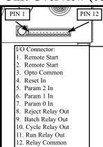
The 12 pin connector on the back of the unit contains several input and output functions.
